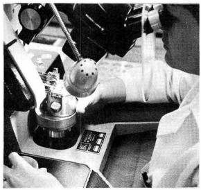
TECHNICIAN Mary Ellen Puckett (2141) attaches 1 mil aluminum wires to a silicon IC die and ceramic package. A microscope is required to position the wires which are ultrasonically bonded.
